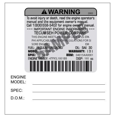
Figure 4. Engine Identification Decal
